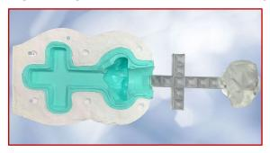
RAMPF silicones are perfect for mold making, rapid prototyping, theming and amusement parks as well as hobby and art projects. The high-performance resin systems exhibit high tear strength, low viscosity, and minimal shrinkage. The easy-to-mix silicones (10:1) are processed via hand batch at room temperature. Shore hardness ranges from 25 to 60A.
