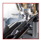
RAMPF adhesives based on polyurethane, epoxy, and silicone combine the ultimate in adhesion and strength with excellent temperature and chemical resistance. They are specifically formulated to provide strong, durable bonds that withstand the rigors of automotive applications.
